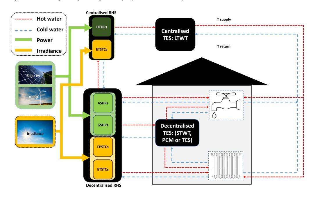
Two-stage modelling approach adopted to determine heat transferred to/from storage on an hourly basis.
